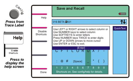
Label Shortcuts Enabling shortcuts allow you to select a column by pressing the key corresponding to the column number. When shortcuts are enabled, press the number key once to move the column, and twice to enter a number.
