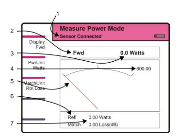
1. Sensor Status Indicates the connection status of the power sensor. 2. **Primary Measurement** Identifies the measurement displayed on the analog dial. 3. **Primary Value** Numeric display of the primary value. 4. Indicates the dial's full scale. **Measurement Scale** 5. Dial Graphic display of the primary measurement. 6. **Secondary Measurements** Identifies measurements not displayed on the dial.
