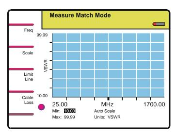
Auto Scale Auto Scale automatically sets the display scale so that the entire trace is displayed.
